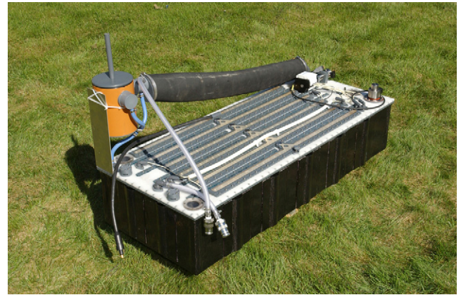
Fig. 1. The Al/HP semi-fuel cell stack with gas separation system and connections.
