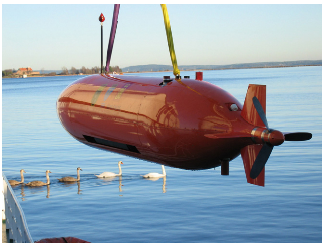
Fig. 7. The last AUV in the HUGIN family: the HUGIN 1000 mine reconnaissance system. The Royal Norwegian Navy has been operating HUGIN 1000 with polymer batteries since February 2004.
